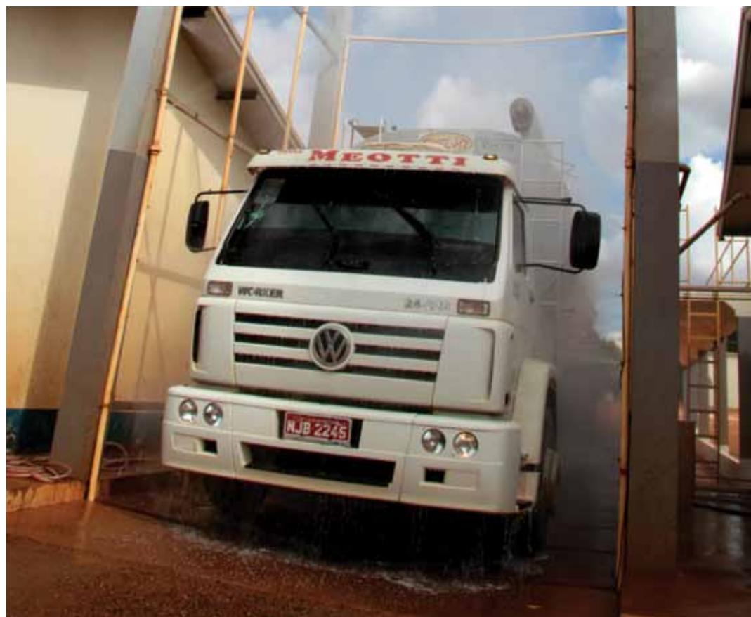
Washing and disinfecting vehicles: greater sanitary control has driven the evolution of the Brazilian poultry industry
